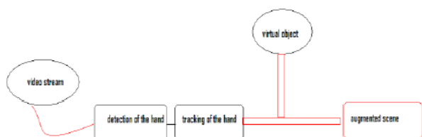
Fig 9: The architecture's of augmented reality system without markers on base of hand
